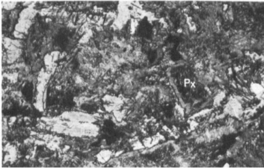
Fig. 3. Unfoliated metadolerite of dike 'M'. Pyroxene (Px) is largely replaced by amphibole. Photomicrograph is 1.3 mm long. Plane light.
