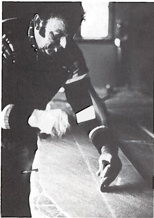
Fig. 3. Quarryman cracking flagstone slab along scored line.
